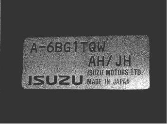
The label to the above left indicates engine model 4BG1 and specification TPW. The AE/JJ indicates a production date of 04/99 (April 1999). The label to the above right indicates engine model 6BG1 and specification TQW. AH/JH indicates a production date of 07/97 (July 1997).
